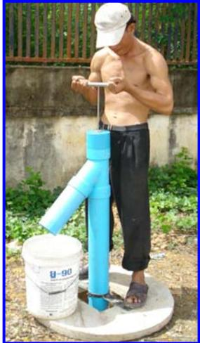
The **GULPER** is designed after inspiration from Tanzania and is used for removing sludge from small septic tanks, wet pit latrines and drain interceptor tanks. Operators don’t have to climb in and/or use buckets and spades; which is common practice in Cambodia. Outside the urban areas there are hardly any sewage systems and a limited number of people have access to sanitation
