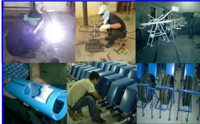
95% of the pumps are fitted on hand dug wells, this is our standard pump which has a depth of 8 meter (vertical), but is capable of being extended much deeper. This year we have also improved the design of our 'pond' pump (diagonal) and a 'school' variety (2-handles for children to use). The pond pump is used by several NGOs. Also we are working on deeper level pumps up to 50 meter deep, irrigation and pedal versions of the pump.
