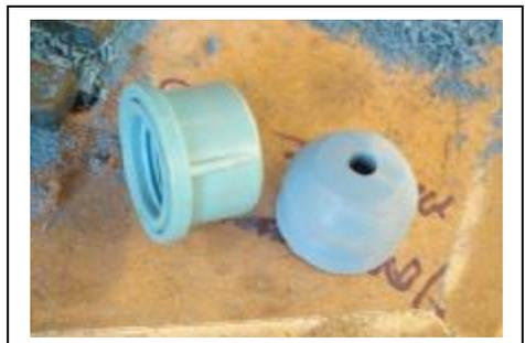
**Figure 5** Original 'end cap' on left and finished 'piston' on the right
