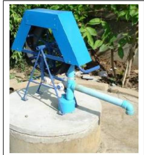
**Figure 3** The pump frame is made from widely available steel stock
