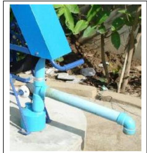
**Figure 4** Standard PVC fitting are assembled in to one unit for the upper guide box and outlet
