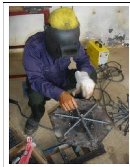
Figure 2 Example of a fixture used during welding the wheel spokes
