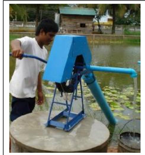
**Figure 12 The 'Pond Rovai' pump fitted at an orphanage in Kompong Thom**
